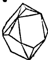
Fig. 165. A figure bounded by 24 faces, of which six are isosceles triangles, twelve scalene triangles, and six pentagons.
